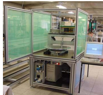
Figure 1: Setup for quality control of niobium sheet material for SNS.
