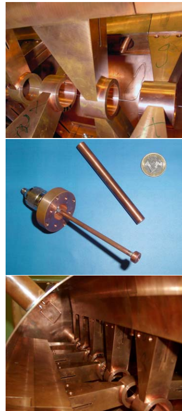
Figure 3: Capacitive coupling through one girder between two stems in the same plane (upper), Capacitive Couplers for the measurements at the copper-model (middle) and Inductive coupler at the CH-Copper-model (lower).
