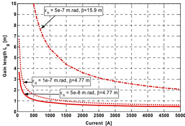
Figure 5: Gain length versus peak current for an undulator period of 8 mm and 0.95 T peak field. Continuous line  $\epsilon_n = 5 \cdot 10^{-8}$ , dotted line  $\epsilon_n = 1 \cdot 10^{-7}$ , dash dotted line  $\epsilon_n = 5 \cdot 10^{-7}$ .
