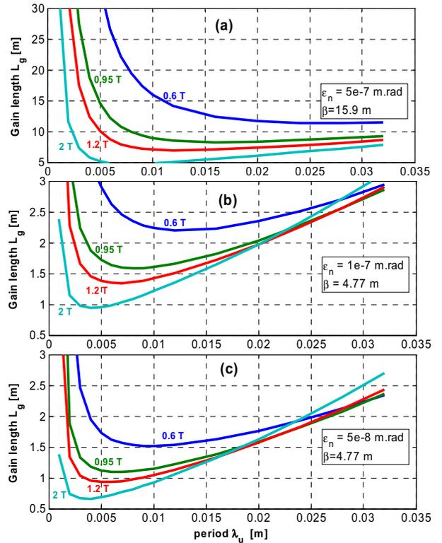
Figure 3: Gain length vs. undulator period for different peak magnetic field and emittances: (a)  $\epsilon_n = 5 \cdot 10^{-7}$  mrad, (b)  $\epsilon_n = 10^{-7}$  mrad, (c)  $\epsilon_n = 5 \cdot 10^{-8}$  mrad.
