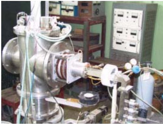
Figure: 6 ECR ion source on the test bench.
