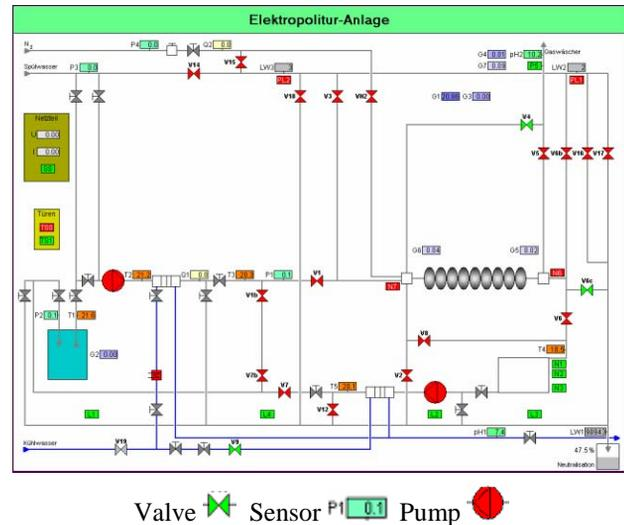
Figure 1: Flow chart of the DESY electro polishing infrastructure.
