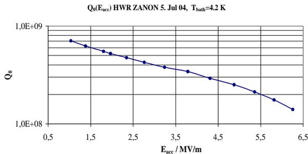
Figure 6: First Q<sub>0</sub>- versus E<sub>acc</sub> measurement.
