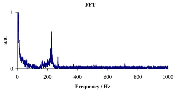
Figure 8: Fast Fourier Transformation of phase-detector signal as response to a 50V step function at the piezos.
