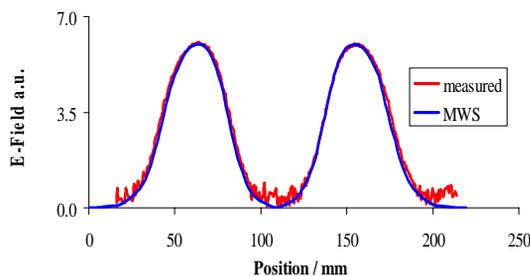
Figure 3: Field profiles, measured and calculated.
