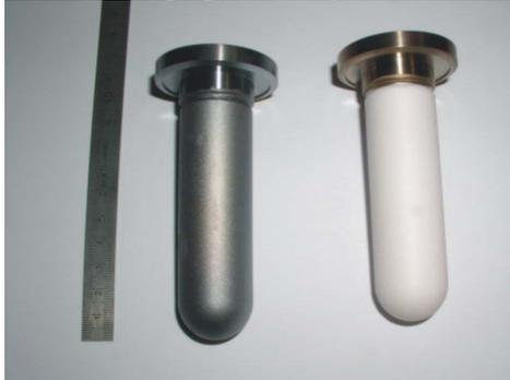
Figure 4: Cold window before (right) and after Ge plating.
