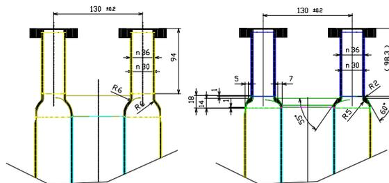
Figure 2: Different end-plate geometries of the HWRs.
