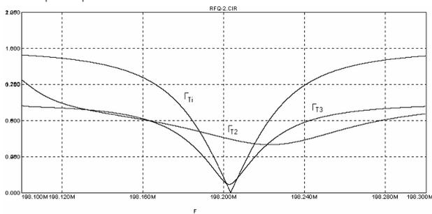
Figure 4: Reflection coefficients as a function of frequency
