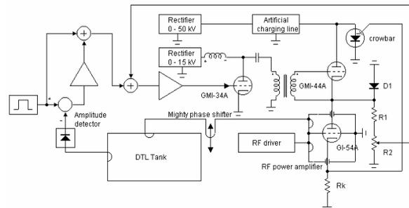
Figure 1: Common view of the DTL RF channel
