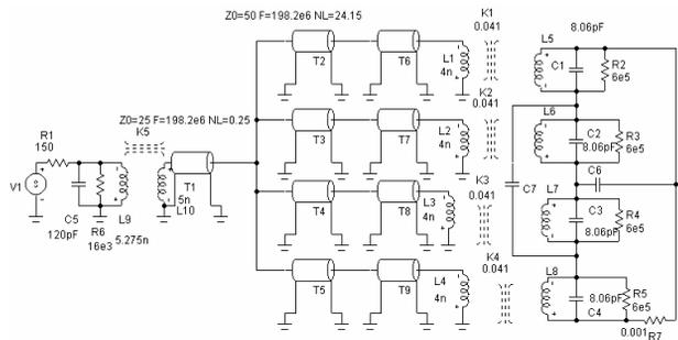
Figure 3: The RFQ RF system supply of their behavior during heating. And indeed, during long beam sessions gradual decrease of RF amplitude in RFQ, accompanied by heating one of the cables, was observed. Attempts to restore the cavity RF amplitude resulted in further increasing of heating of the cable and breakdowns in the area of the RFQ coupling loops. For estimation of processes in cables, modeling of the RFQ
