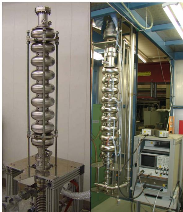
Figure 2: TESLA Cavities for BESSY during HPR at ACCEL (left) and vertical testing at DESY (right).
