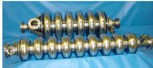
Figure 1: SNS (upper) und TESLA (lower) Cavity.
