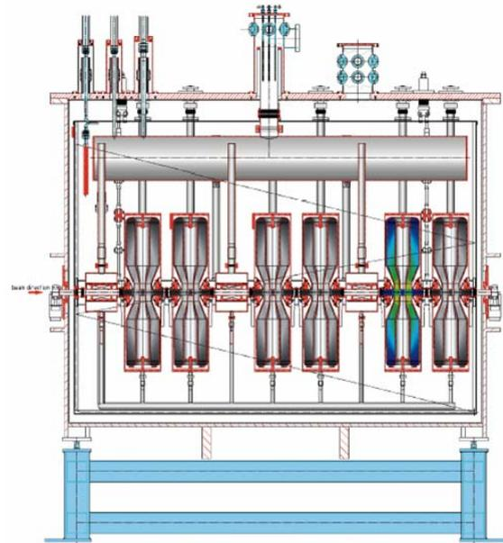
Figure 11: Scheme of the prototype SRF module for SARAF with 6 bulk niobium HWR and 3 superconducting solenoids. The beam vacuum is separated from the cryostat vacuum.
