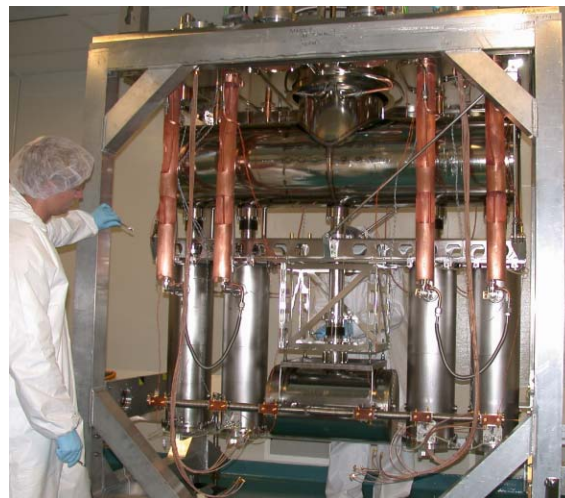
Figure 1: Cryomodule top assembly in the assembly frame prior to the cold test.
