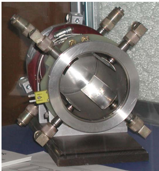
Figure 1: IPNS 50 MeV line stripline BPMs.
