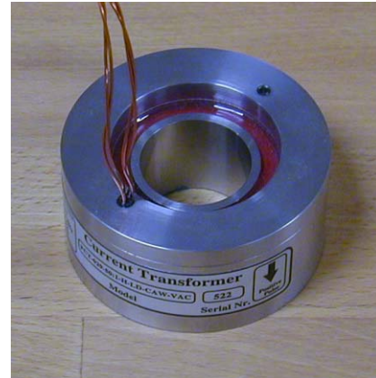
Figure 1: SNS transformer for the DTL section.
