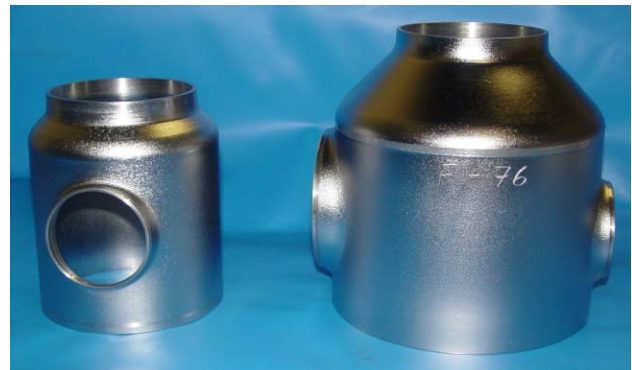
Figure 1: Raw end groups produced for SNS cavities by deep drawing and nipple pulling from one reactor grade niobium sheet.
