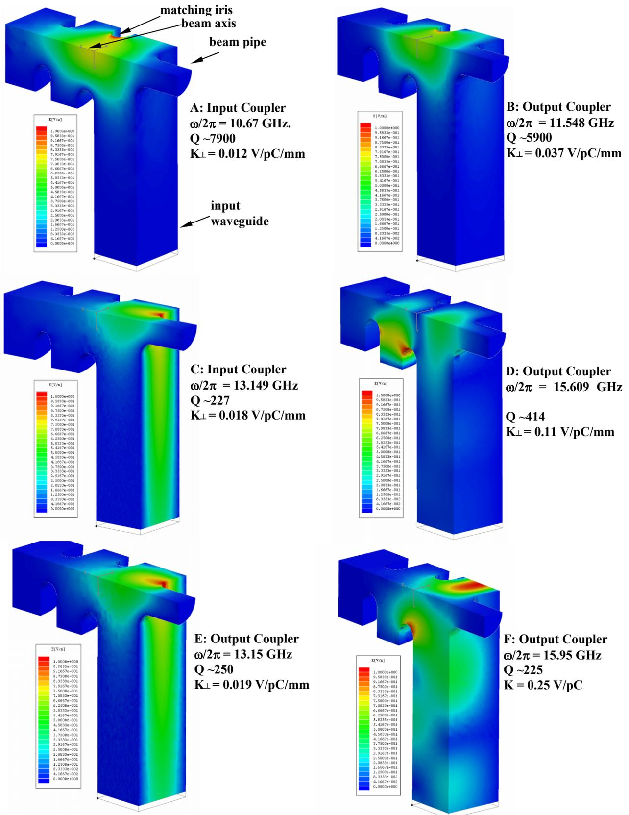
Figure 1: Surface electric fields of the trapped modes in the input and output fundamental couplers of the accelerator structure known as H60VG4S17-III-SN2. The resonant frequency ( $\omega/2\pi$ ), Q value and the dipole mode kick factor ( $K_{\perp}$ ), are indicated except for the monopole-like mode in F, where the monopole loss factor ( $K$ ) is indicated. One quarter of the geometry was simulated with appropriate boundary conditions.
