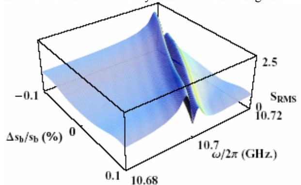
Figure 3: Surface of  $S_{RMS}$  (V/pC/mm/m), the RMS of the sum wakefield in the vicinity of the peak value. The trapped mode frequency is given by  $\omega/2\pi$  and,  $\Delta s_b/s_b$  is the fractional change in the bunch spacing from 1.4 ns. The large peaks occur close to harmonics of the bunch frequency (714 MHz at the nominal bunch spacing).
