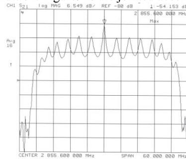
Figure 7: The dispersion relation of the tube
