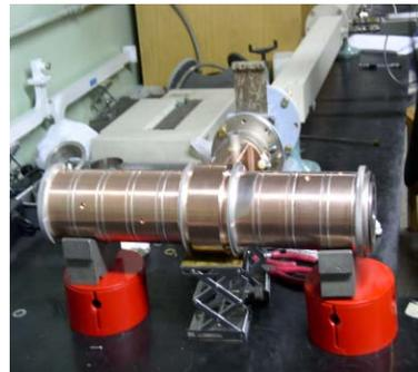
Figure 9: The accelerating tube
