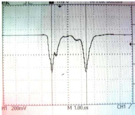
Figure 4: Waveform, reflected power at accelerator Guide resonance.
