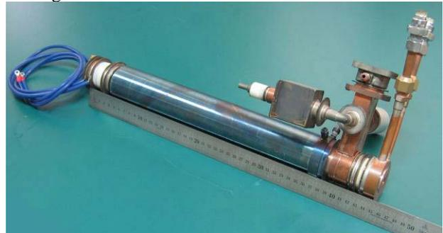
Figure 1: The accelerating guide after brazing.
