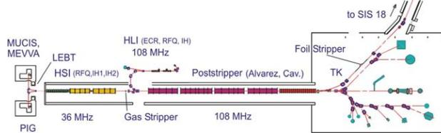
Figure 1: Schematic overview of the GSI UNILAC.
