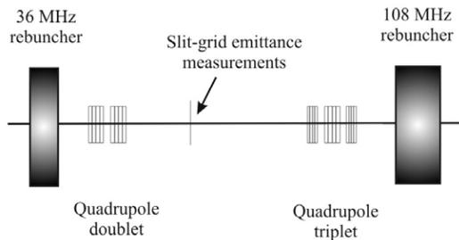
Figure 3: Matching section to the 1<sup>st</sup> Alvarez DTL.
