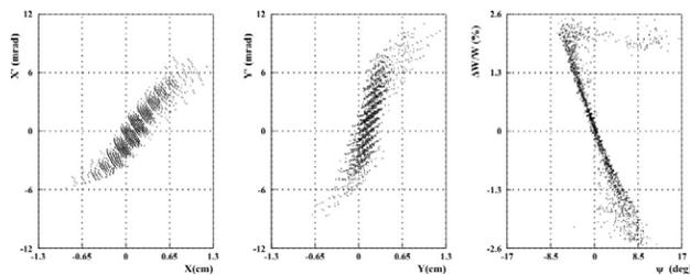
Figure 6: The particle distribution at the entrance of the 1<sup>st</sup> Alvarez tank simulated with the DYNAMION code from the position of emittance measurements.
