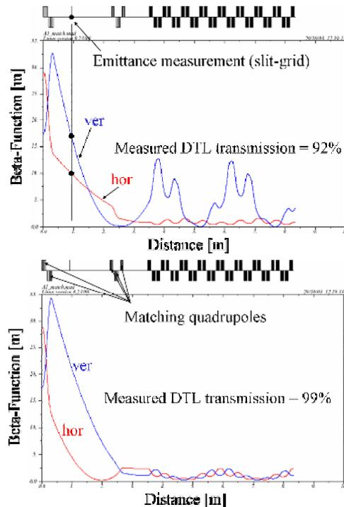
Figure 5: Horizontal and vertical beta-functions in the matching section and first cells of the 1<sup>st</sup> Alvarez tank with quadrupole setting before (upper graph) and after (lower graph) optimization.
