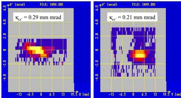
Figure 6: Normalized emittances from the IH-structure. A 1nA He<sup>+</sup>-beam has been used for the measurements.
