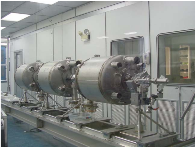
Figure 2. SNS \beta=0.61 three-cavity string assembled in the clean room. Indium seals were used in this prototype while more efficient seals are being developed for production.
