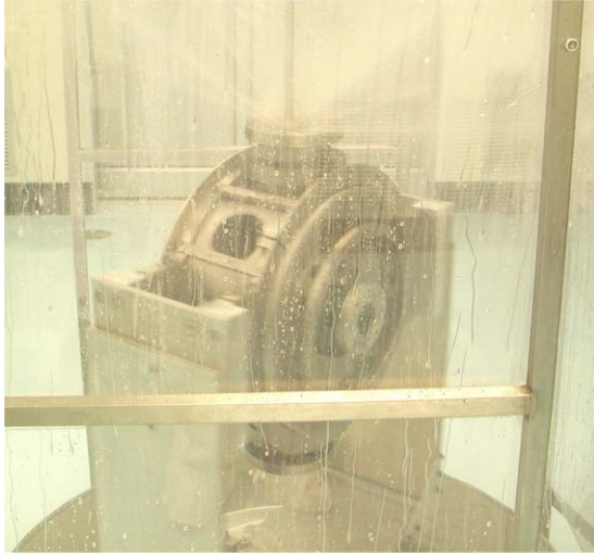
Figure 2: The cavity being high-pressure rinsed with ultra-pure water at ~1200 psi. The cavity rotates at ~ 23 rpm and the HPR wand sweeps the cavity vertically at 3.9 mm/s (up) and 7.5 mm/s (down).
