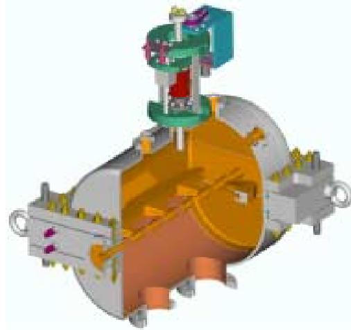
Figure 4: Design study of one of the real IH-7-gap resonators
