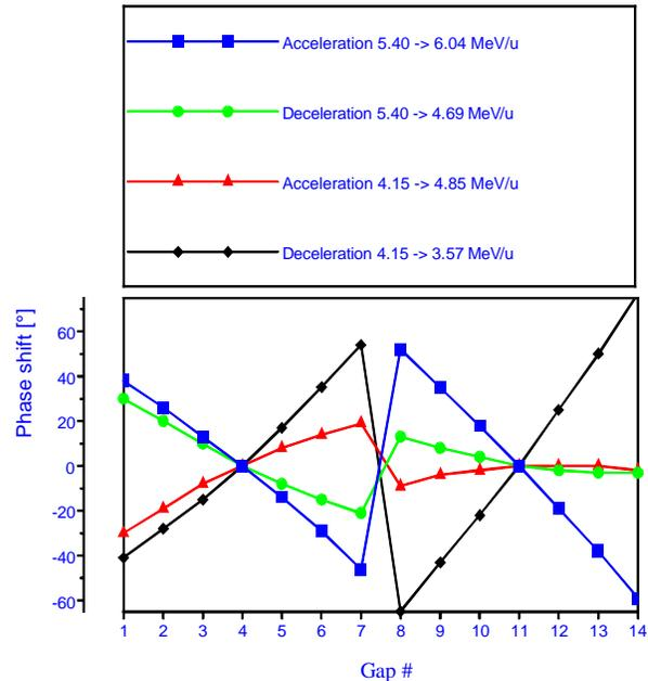
Figure 2: Phase shift of the ion bunch in relation to the synchronous particle
