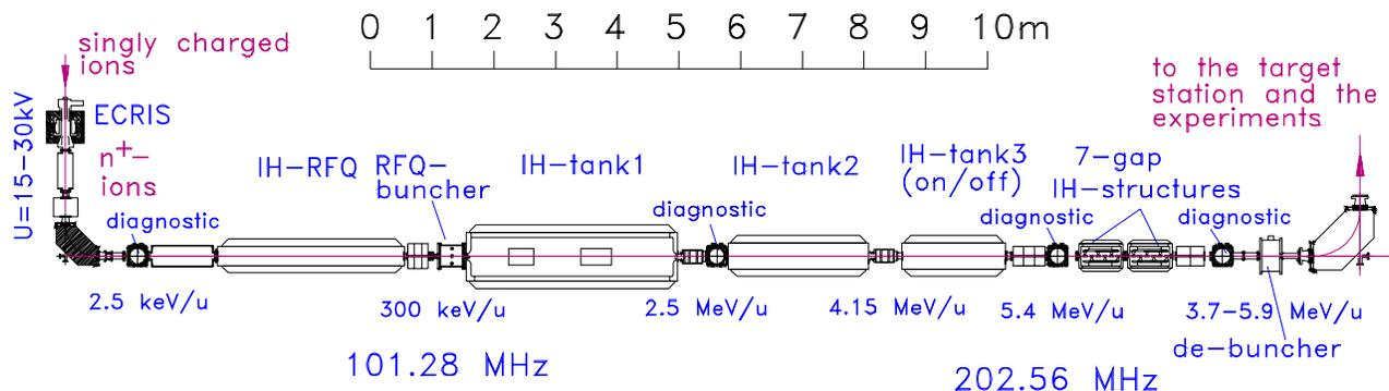
Figure 1: Layout of the MAFF LINAC. The overall length is limited to 20 m due to the experimental hall. The final energies can be varied between 3.7 MeV/u and 5.9 MeV/u via two 7-gap-IH resonators.
