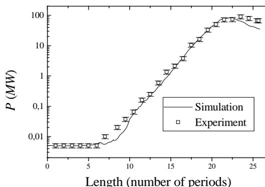
Figure 1: Comparison between experimental and calculated power growth in the wiggler.
