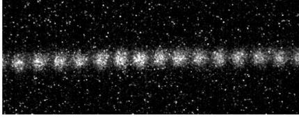
Figure 2: Example of a streak camera image showing 14 bunches at 35 GHz.
