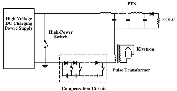
Figure 1: Basic line-type modulator with a compensation circuit.
