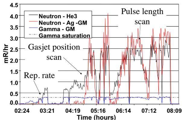
Figure 4: Neutron and Gamma production as a function of time illustrates repeatable, controllable, high energy electron beam production.
