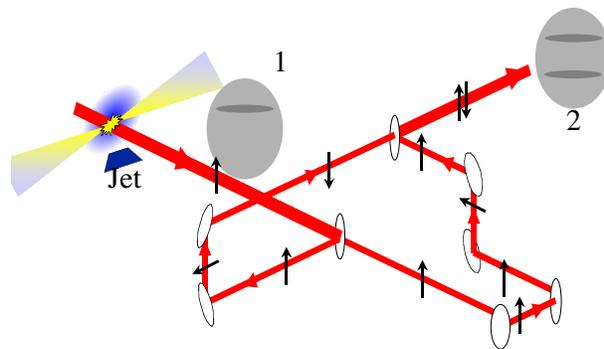
Figure 3: Lay-out of the folded wave interferometer used for measuring the plasma density profile. A single image of the interaction region at (1) is split, folded, and recombined to form two interfering images at the detector (2).
