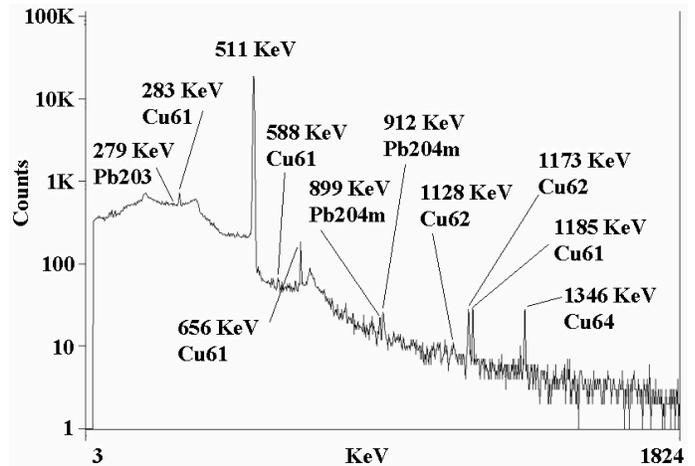
Figure 9: Example gamma ray spectrum from the nuclear activation measurements, showing the peaks corresponding to each isotope produced.
