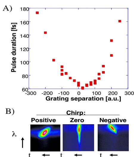
Figure 2: (a) Laser pulse duration vs. compressor grating separation. (b) Spectrum vs. time measured using a frequency resolved optical gating system. The laser chirp sign changes as the pulse compression crosses its minimum value.
