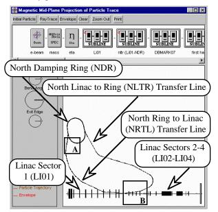
Figure 1. Layout of the SLAC linac sectors, the north (electron) damping ring, and the associated transfer lines.
