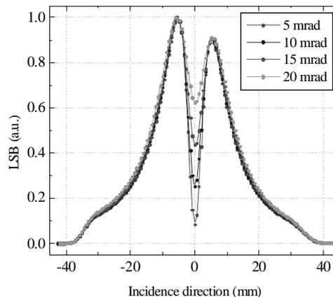
**Figure 4: Simulations of the effect of the divergence angle on the OTR angular distribution (20 MeV).**
