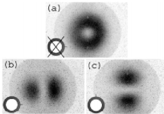
**Figure 3: Experimental picture of the OTR polarisation. The beam energy is 3.8 MeV**
