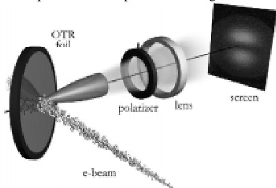
**Figure 2: Experimental set-up for angular distribution measurement.**
