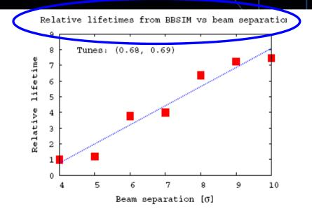
Figure 5: Relative lifetime vs separation with BBSIM.
