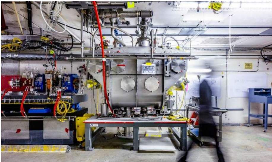
Bunch lengthening system in Zone F
