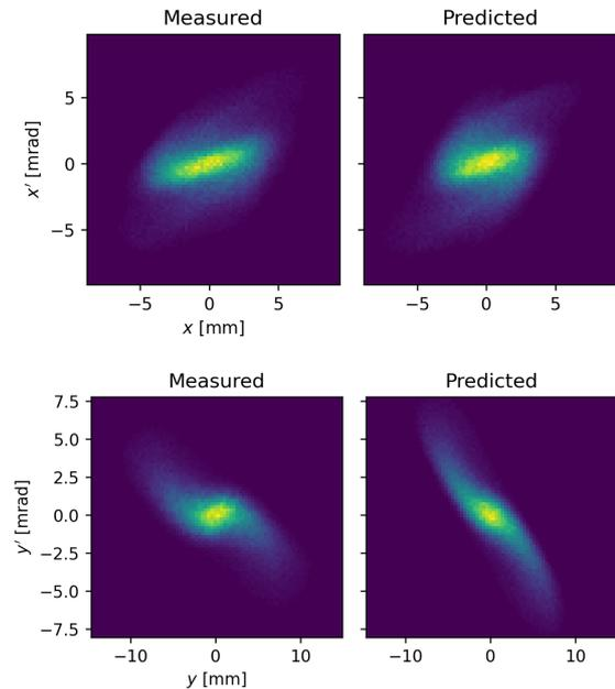
Figure 4: Beam phase space at end of beam-line.
