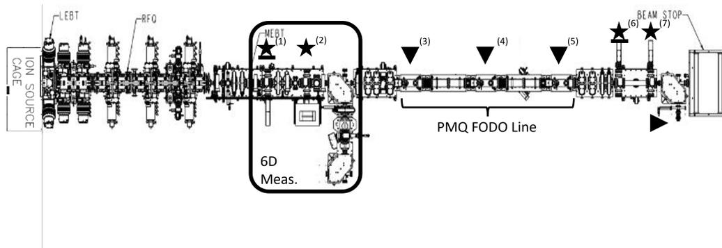
Figure 1: Layout of straight BTf configuration. The symbols represent diagnostic locations. Triangles: intensity limited profiles. Stars: profiles. Underlined Stars: phase space. Box: 6D measurements. Note: at each star there is a set of both horizontal and vertical slits.
