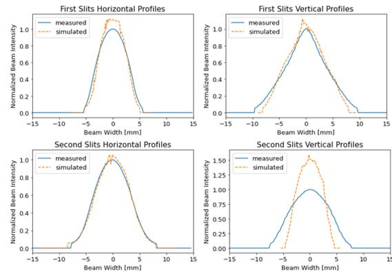
Figure 3: Beam profiles at end of beam-line.
