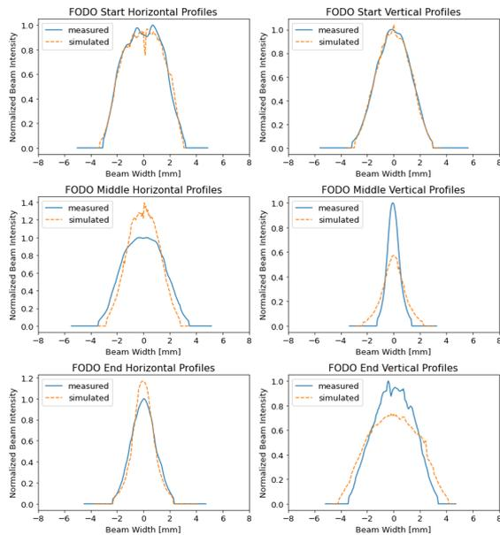
Figure 2: Beam profiles at each of the screens within the FODO line.
