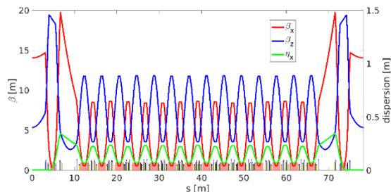
Figure 2: New booster optical functions (half ring).
