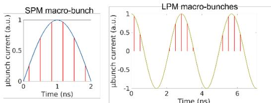
Figure 4: Linac beam time structure at booster entrance with its 3 GHz  $\mu$ -bunches in SPM mode (1 to 4 macro-bunches) and LPM mode (104 macro-bunches).
