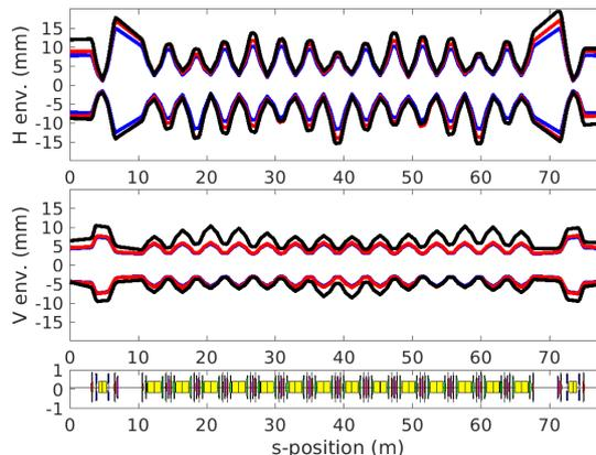
Figure 6: Beam envelopes at injection for an emittance  $\epsilon_{n90\%}=100 \cdot 10^{-6} \pi$  m.rad and (red) the ideal lattice w/o coupling (blue) the ideal lattice w/ 99% coupling and maximum  $f_{RF}$  shift (black) the lattice w/ all errors giving the minimal D. A. Only half booster is represented.
