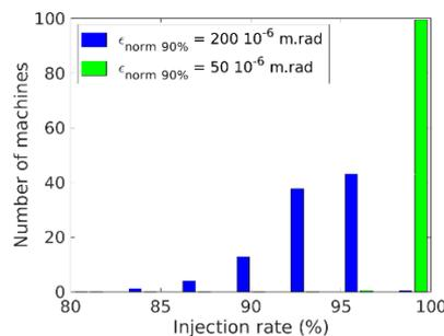
Figure 7: Injection rate of the SPM macro-bunch from LTB transfer line into the booster, w/ an elliptical aperture  $H36 \times V22$  mm<sup>2</sup>, considering the worst booster D.A. and all injection errors in 100 seeds.
