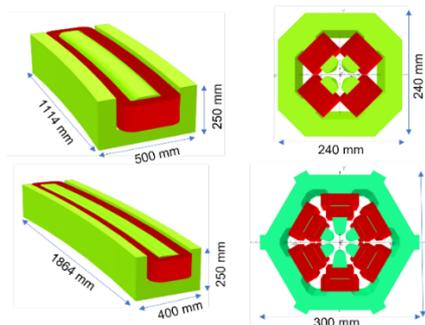
Figure 8: Booster new magnet design for short and long dipoles, quadrupole and sextupole.
