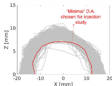
Figure 3: On momentum dynamic aperture of the SOLEIL II booster in presence of all errors (300 seeds), calculated at the middle of the long straight section.
