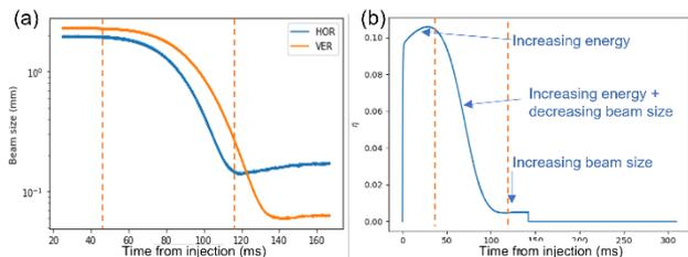
Figure 1: (a) Foreseen beam sizes along the booster ramp and (b) ion neutralization factor of day 1 w/ a total pressure of  $3.10^{-6}$  mbar and in presence of 1 nC/s.
