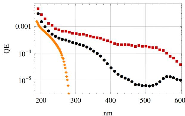
Figure 3: The quantum efficiency (QE) of a thermionic dispenser cathode was measured for different wavelengths of the illuminating source. Measurements are compared for the unheated (black) and heated (red) operation. The results are compared to the quantum efficiency of a copper cathode (orange) (from Ref. [3]).
