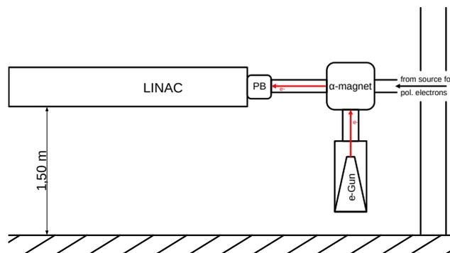
Figure 2: Schematic drawing of the transfer beamline connecting the electron sources to LINAC2.
