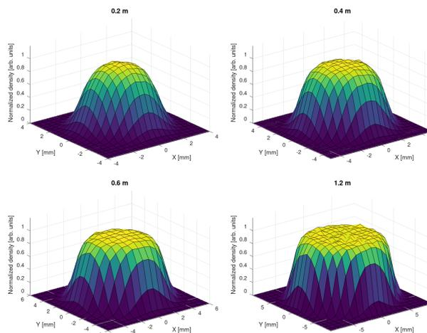
Figure 2: Evolution of the transverse beam distribution along the injector from a Gaussian distribution at the cathode. Corresponding kurtosis values are  $k_{x,y}=2.36 / 2.34$  at 0.2 m,  $k_{x,y}=2.20 / 2.22$  at 0.4 m,  $k_{x,y}=2.13 / 2.15$  at 0.6 m, and  $k_{x,y}=2.05 / 2.05$  at 1.2 m.
