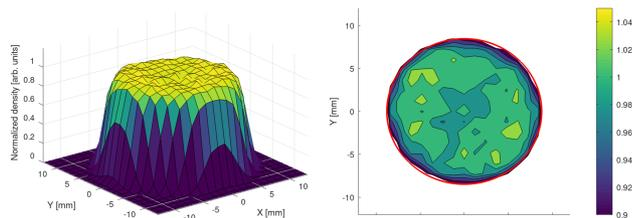
Figure 1: Simulated uniform distribution at 1.8 m from the cathode for 0.17 T magnetic field: (left) histogram of the particle distribution and (right) colour map representation. Corresponding kurtosis values are  $k_x=2.027$  and  $k_y=2.022$ .
