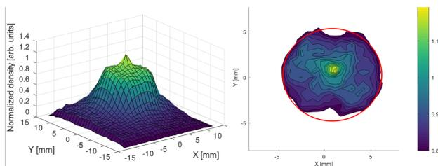
Figure 5: Experimentally measured particle distribution for a solenoid field of 0.153 T at BTv215: (left) histogram of the particle distribution and (right) colour map representation
