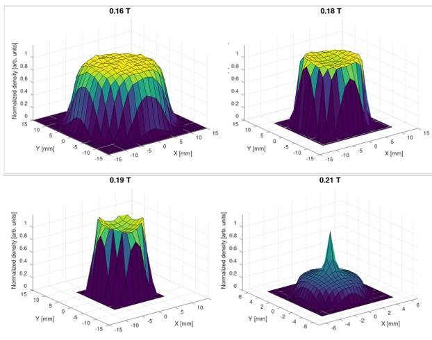
Figure 3: Effect of the magnetic field variations near the first and second uniformity points at 180 cm. Corresponding kurtosis values are  $k_{x,y}=2.07$  for  $B=0.16$  T,  $k_x=1.98$ ,  $k_y=2.00$  for  $B=0.18$  T,  $k_x=1.99$ ,  $k_y=1.95$  for  $B=0.19$  T, and  $k_x=2.19$ ,  $k_y=2.21$  for  $B=0.21$  T.
