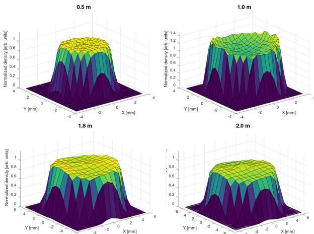
Figure 4: Simulation results for the magnetic field of 0.2 T optimised to reach the second uniformity point at 180 cm. Corresponding kurtosis values are  $k_{x,y}=2.04 / 2.04$  at 1.0 m,  $k_{x,y}=1.93 / 1.97$  at 1.0 m,  $k_{x,y}=1.99 / 2.03$  at 1.8m, and  $k_{x,y}=2.0 / 2.05$  at 2.0 m.
