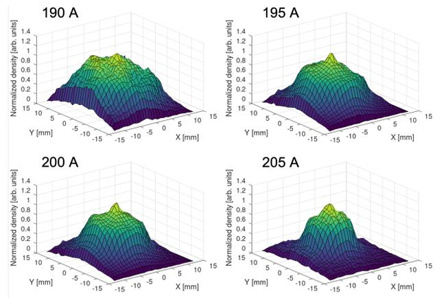
Figure 6: Experimentally measured particle distributions at BTv215 for different current settings in the FC: 190 A, 195A, 200 A, and 205 A. The BC current was adjusted accordingly to keep the zero magnetic field at the cathode. The corresponding peak solenoid field is varied within 0.14-0.153 T.
