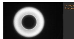
Figure 5: Electron beam from the HEL gun, with 100 mA and 3  $\mu$ s pulse. The round and uniform structure of the beam is clearly visible.
