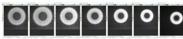
Figure 6: HEL gun electron beam, imaged at the YAG screen, during magnetic compression with 20 mA and 3  $\mu$ s pulses. The outer beam diameter (in mm) is, from left to right, 24, 26.5, 24.4, 21.6, 19, 17.1 and 13.2. The beam moves during compression indicating a slight misalignment of the gun with respect to the axis of the magnetic field lines. The misalignment was corrected for later measurements.
