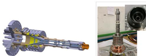
Figure 4: HEL electron gun [9] 3D model (left) and prototype (right). The hollowed cathode has an inner and outer diameter of  $\sim 8.05$  mm and  $\sim 16.10$  mm respectively, and can be seen in the enlargement inside the anode.
