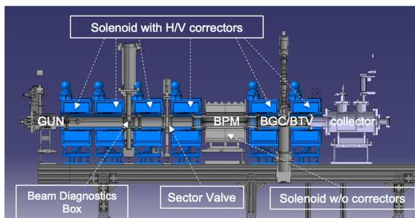
Figure 1: Schematic of the CERN electron beam test facility.
