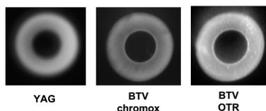
Figure 7: YAG, Chromox and OTR screen images. The shots parameters were respectively: 364 mA, 4.6 keV, 5  $\mu$ s; 2 mA, 7 keV, 5  $\mu$ s; and 1.2 A, 7 keV, 25  $\mu$ s.
