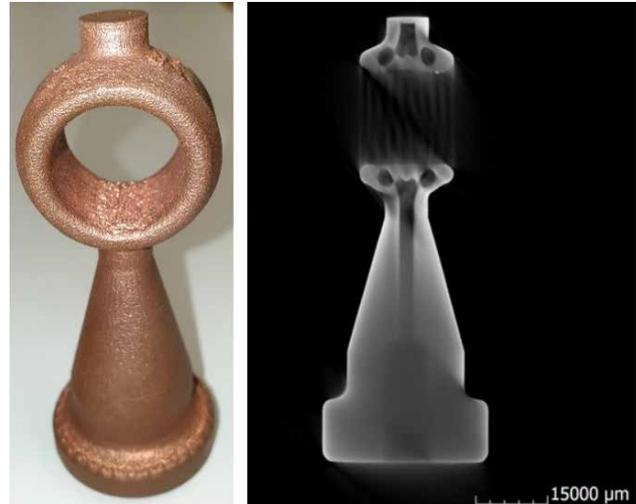
Figure 4: CH electrode model printed with copper (left) and checked with Computed Tomography (right) [8].
