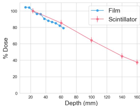
Figure 3: Comparison between doses measured by the PSDs and by the radiochromic films.
