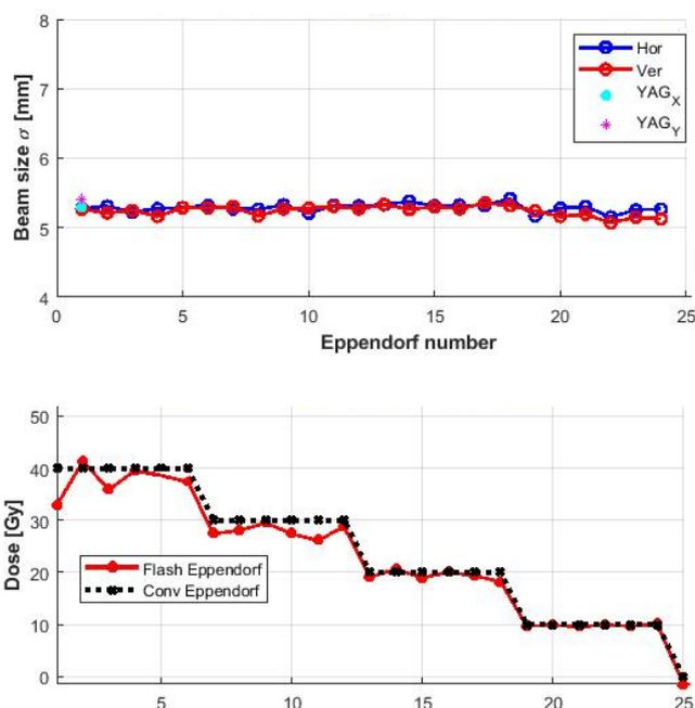
Figure 6: Measured beam sizes and delivered doses for CHUV chemistry studies.
