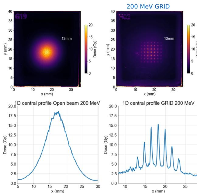
Figure 1: Beam profiles from the radiochromic films without (left) and with (right) the tungsten grid collimator inserted.
