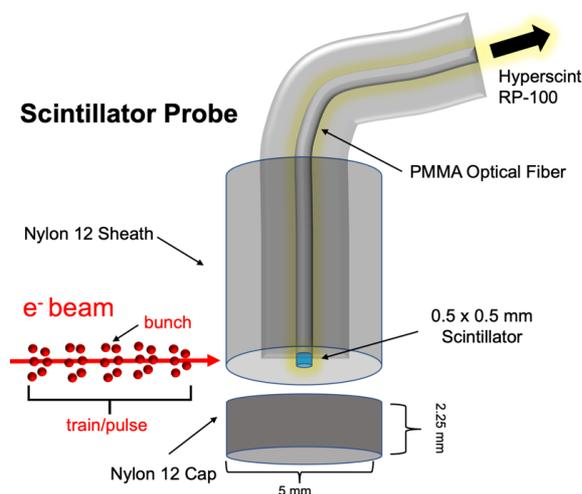
Figure 2: Schematic of the scintillator probe.
