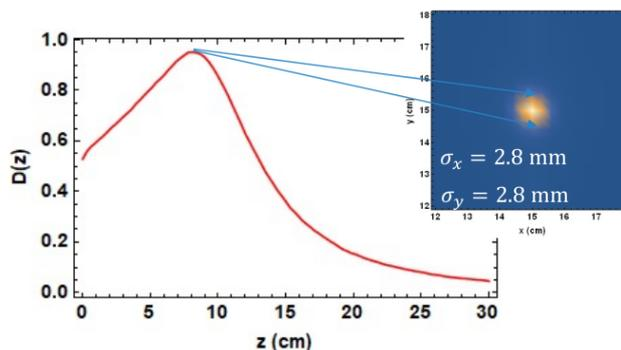
Figure 4: Simulation of the relative delivered dose deep in a water phantom.
