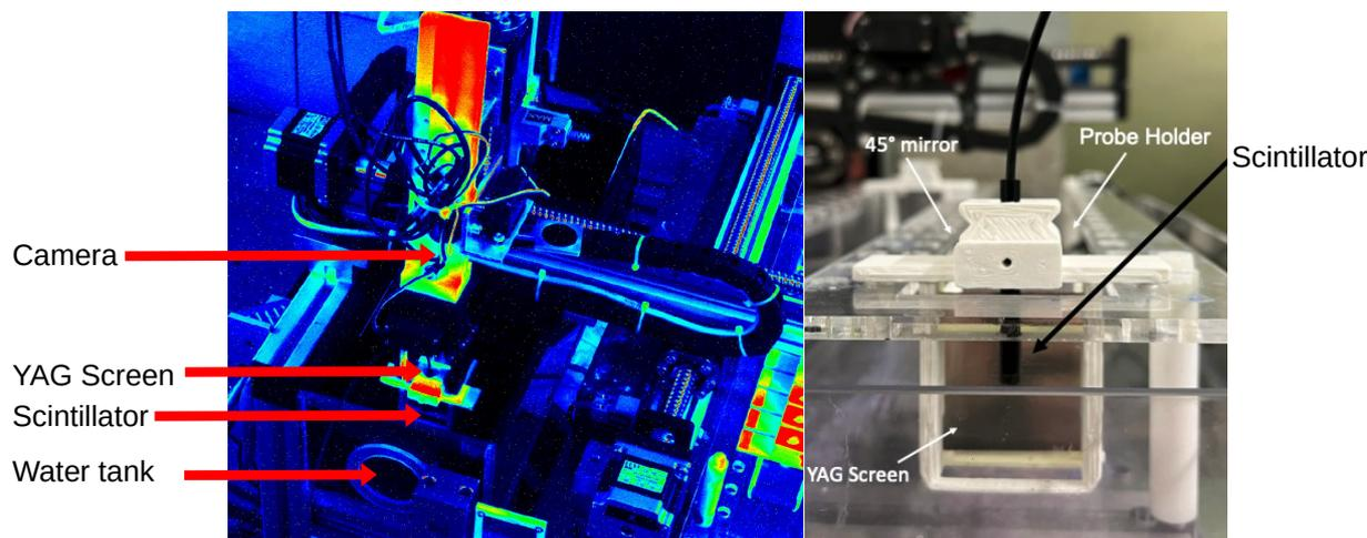
Figure 5: Scintillator and YAG screen in the electron beam (left), 3D printed holder with the scintillator and the YAG screen (right).
