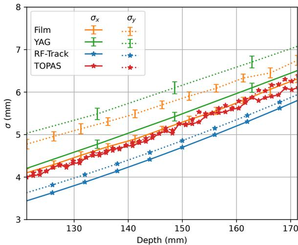
Figure 4: The evolution of the  $1\sigma$  beam size as a function of depth, as measured by the films and YAG screens irradiated under CONV conditions.
