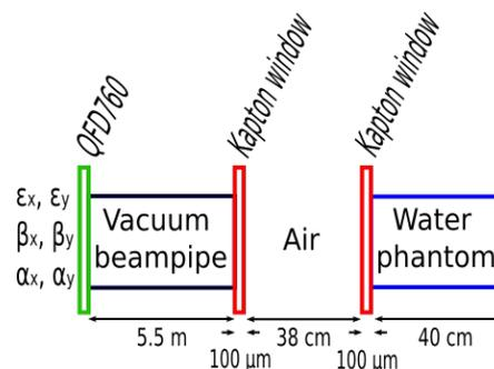
Figure 3: A schematic of the experimental setup. QFD760 refers to the entry of the quadrupole used as reference for the quadrupole scans.
