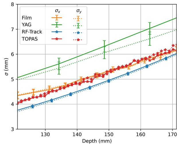
Figure 5: The evolution of the  $1\sigma$  beam size as a function of depth, as measured by the films and YAG screens irradiated under FLASH conditions.
