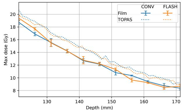
Figure 6: The evolution of the maximum dose as a function of depth, as measured by the films irradiated under both CONV and FLASH conditions.
