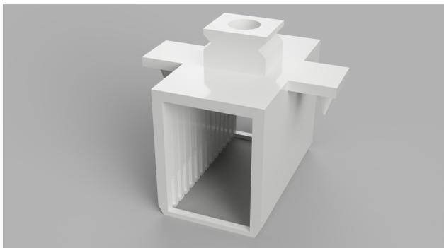
Figure 2: Robot holder for in-water film irradiations. It has a total of 14 slots placed  $\sim 5$  mm apart, each having the capacity of holding 3 films placed back-to-back.
