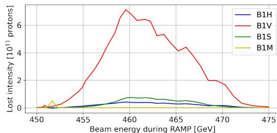
Figure 2: Proton impacts on the B1H (horizontal), B1V (vertical), B1S (skew) and B1M (off-momentum) primary collimators around a beam lifetime drop at the beginning of the energy ramp.
