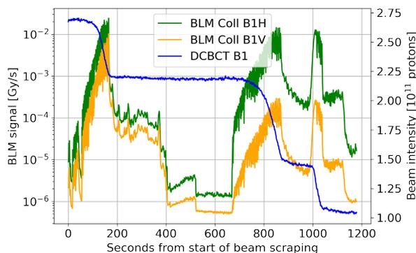
Figure 1: Beam 1 intensity measured with the DCBCT and BLM signals at primary horizontal and vertical B1 collimators during B1 vertical and horizontal beam scraping.
