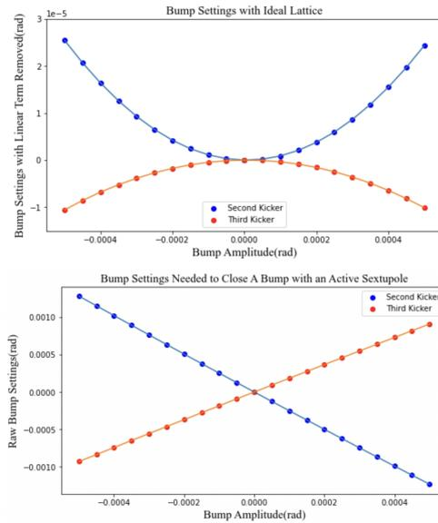
Figure 3: second and third corrector data with linear term removed (Top) and without linear term removed (Bottom) in an ideal lattice without BPM errors. Not that the extrema of the parabola are at the origin, because the sextupole was not misaligned in this example.
