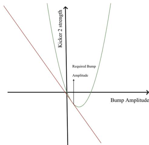
Figure 2: Strength of corrector-2 that closes the 3-bump with (green parabola) and without (red line) a sextupole as a function of the bump amplitude, which is created by corrector-1. The two curves meet when the orbit is in the center of the sextupole.
