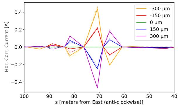
Figure 4: Measured (solid) and simulated (dotted) horizontal corrector currents for the five girder positions as a function of the corrector location counted from the East symmetry point in anti-clockwise direction. Corrector magnets are displayed as small dark blue elements in Fig. 2. Values are given relative to the original girder position.
