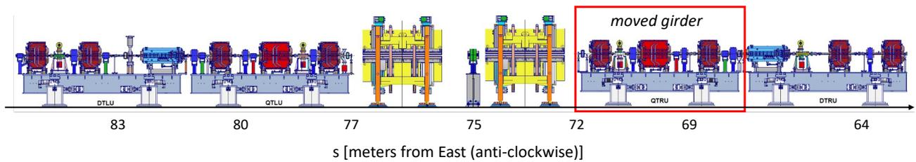
Figure 2: Graphical view on the accelerator elements in the proximity of the moved girder (marked with red rectangle). Location numbering is given from the East symmetry point of the PETRA III ring counting anti-clockwise (towards the left, viewed radially outward from the centre of the ring).
