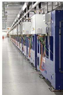
The row of U15 undulators for the ARAMIS beamline at the SwissFEL at PSI [5]
