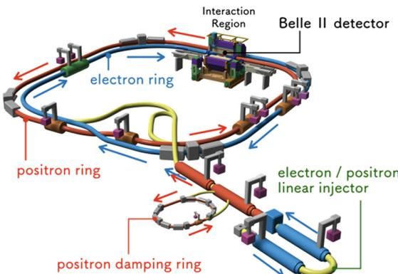
SuperKEKB is an asymmetric-energy e+e- collider based on the “nanobeam scheme, where two low emittance beams collide with a large crossing angle at the IP.
