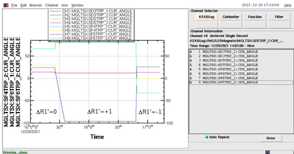
We tested tilting the magnets with keeping the beam at the end of this study and found no problem (no sudden loss of the beam, no sudden change in the beam orbit and so on).
