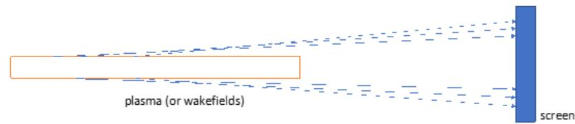
Defocused protons leave the plasma before SM reaches saturation
