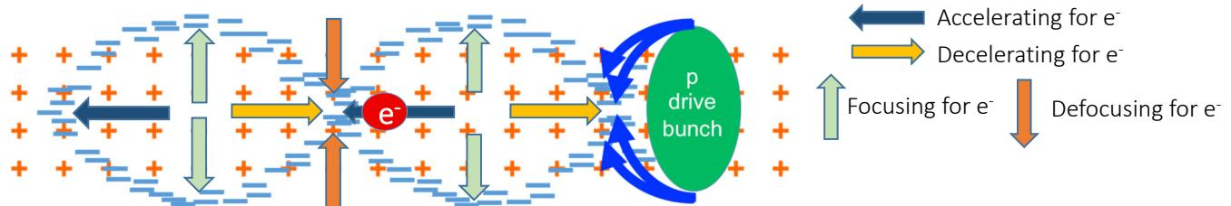
Charged particle bunch traveling inside a plasma perturbs the plasma electron distribution
