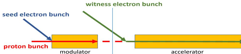
Optimize acceleration of electrons in p-driven plasma wakefield
