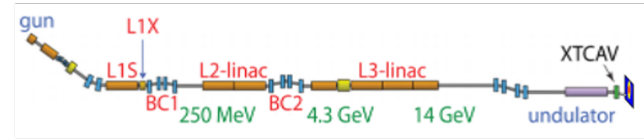
Linac sim in Bmad with collective beam effects
