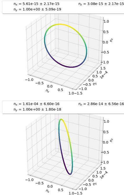
Figure 2: Spin precession plane simulated by tracking the reference particle for  $10^4$  revolutions in an idealized Bmad COSY model. The upper figure displays a simulation without an EDM signal, while the lower figure shows a simulation with an EDM signal of  $\eta = 10^{-4}$  included. The invariant spin axis  $\langle \vec{n} \rangle$  is the vector perpendicular to this plane. Its orientation is displayed in the legend.
