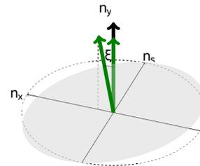
Figure 1: A permanent EDM of magnitude  $\eta$  tilts the invariant spin axis in horizontal direction  $n_x$  by the angle  $\xi$ . The longitudinal direction  $n_s$  is not affected by a permanent EDM.
