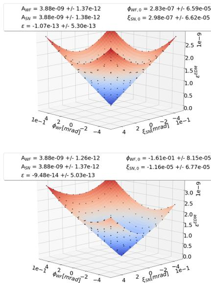
Figure 4: The upper graph shows a simulated resonance map without an EDM contribution, while the lower graph shows a simulated resonance map with an EDM signal of  $\eta = 10^{-4}$ . The x- and y-axis indicate the RF-Wien filter rotation and the solenoid strength, while the z-axis shows the EDM resonance strength. The legend shows the fit parameter when fitting Eq. (5) to the simulated data.
