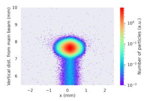
Figure 3: Transverse distribution of protons impacting the target in the proof-of-principle setup. The colour indicates the number of particles.
