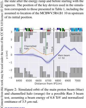
Figure 2: Simulated orbit of the main proton beam (blue) and channelled halo (orange) for a possible Run 3 beam test, assuming a beam energy of 6.8 TeV and normalized emittance of 3.5  $\mu$ m rad.
