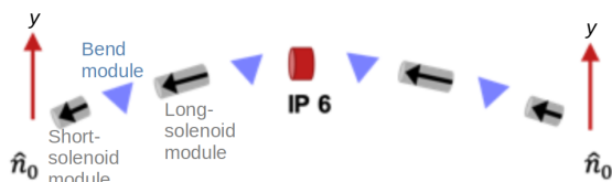
Figure 3: The spin rotators are composed of short- and long-solenoid modules, as well as bend modules, to rotate the spin from vertical in the arcs to longitudinal at the IP and back to vertical on the other side.
