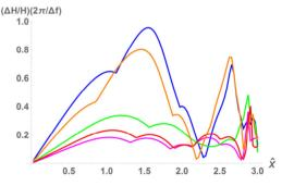
Figure 12: RF-phase ramps in 3 synchrotron oscillations.
