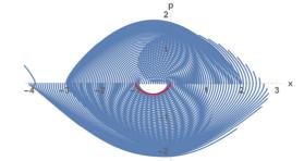
Figure 5: Particle trajectories for linear RF-phase sweep.
