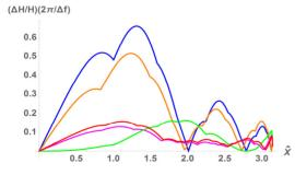
Figure 9: RF-phase ramps in 4 synchrotron oscillations. Conclusions: (1) "linear" is best for n = 1. Also: if linear ramp is used and amplitudes <0.5 radian, then no point using n>1. (2) "Bi-quadratic" is best for n = 2 and amplitudes <2 radian. (3) "½-sine" is best for n = 3. (4) "Bi-quadratic" is best for n = 4 unless amplitudes < 1.5 radian.
