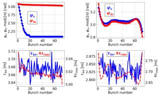
Figure 3: Top: average of the bunch profile (red) and synchronous phase (blue) along the batch at injection (left) and after 0.5 s (right). Bottom:  $\tau_{4\sigma}$  (blue) and  $4\tau_{\rm rms}$  (red) along the batch at injection (left) and after 0.5 s (right).
