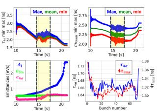
Figure 7: Top and bottom left: same color legends as in Fig. 6. The shaded area indicates the time interval for controlled emittance blow-up. Bottom right: extracted  $\tau_{4\sigma}$  (blue) and  $4\tau_{\rm rms}$  (red) along the batch.
