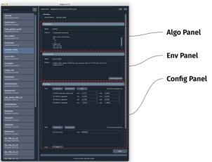
Figure 3: Badger routine editor. With the routine editor, users could select the optimization algorithm and environment to use, change the hyper-parameters for the algorithm and the environment, and configure the variables, objectives, and constraints (VOCs) of the routine.
