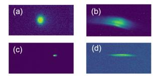
Figure 3: Serialized beam property measurements. (a) beam profile at sample plane (b) virtual cathode (VCC) image (c) beam profile on diffraction detector (d) beam streaked in horizontal using a high field enhancement THz structure, horizontal width corresponds to pulse length.
