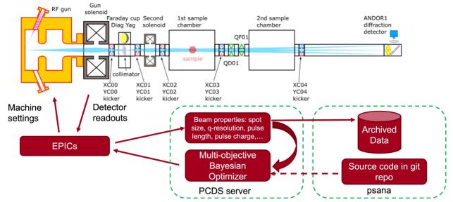
Figure 2: UED beamline layout and MOBO work flow.
