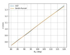
Figure 4: Validation of the THz peaks emitted at different angles from the CST simulation versus the analytical Smith-Purcell equation.
