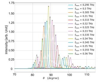
Figure 3: THz radiation spectrum as a function of emission angle obtained by doing a frequency scan at the farfield monitor in CST.
