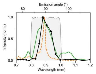
Figure 5: Measured and simulated emission spectrum. Black curve is experimental, orange and green curves are frequency-domain and time-domain simulations [14].
