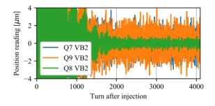
Figure 3: Injection into LHC captured by the old (Q7,Q9) and new (O8) beam pos. meas. module. Data are notch filtered and  $\beta$ -normalized, so they can be directly compared.
