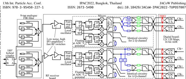
Figure 1: Diagram showing the new receiver topology, with important sub-circuits which influence the overall noise performance. Black lines are 50  $\Omega$  characteristic impedance, blue elements and lines are 100  $\Omega$ .
