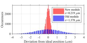
Figure 2: Comparison of position measurement quality for the old and new BeamPos modules (27000 samples). Same operating conditions, such the performance can be directly compared.
