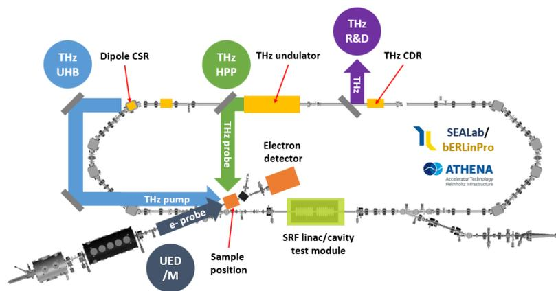
Figure 3: Footprint of the bERLinPro/SEALab accelerator with overlays for multi-color radiation source opportunities.
