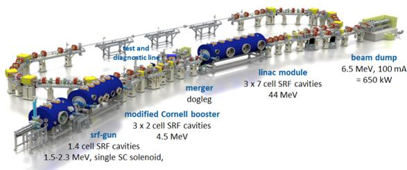
Figure 2: An overview of the bERLinPro/SEALab accelerator.
