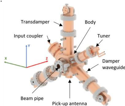
Figure 1: 1.5 GHz cavity, HOM damped with Ridged Circular waveguide and *TransDampers*.
